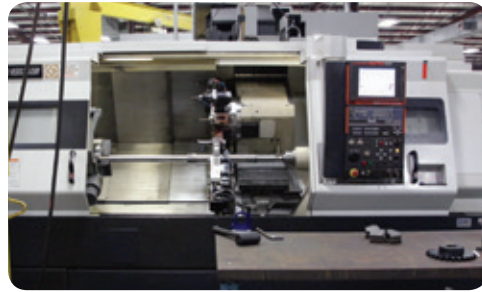
Mazak CNC Lathe with Live Tooling and "Y" Axis (60" between centers, 4.4" through spindle, 12" chuck)
