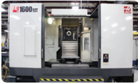
Haas CNC Horizontal Machining Center (64" x 50" x 40") with 4 th axis rotary turntable built in
