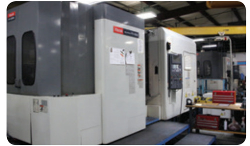
Mazak CNC Horizontal Machining Centers with Pallet Changers (31.4" x 31.4" x 34.6") high torque 6,000 rpm and high speed 10,000 rpm
