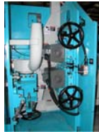
Both End Matcher Stations Equipped with Trim Saw, Top & Bottom Tongue/Bevel/Score And Vertical Groove/Cope
